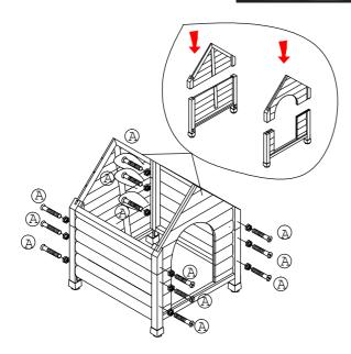
step 1 : secure the front, back and side panels with screws A.
