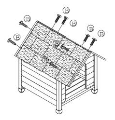
step 3 : attach the roofs with screws B.
